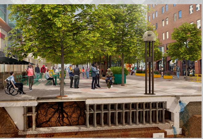
growth and streetscape durability. The project also incorporated Continuously Reinforced Concrete Pavement, typically used on highways, to withstand a high-load transit setting.
